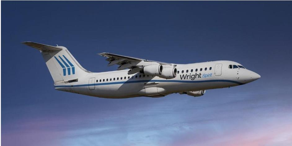
Figure 9 - BAe146 retrofit Wright Electric all-electric aircraft (source: Wright Electric)
