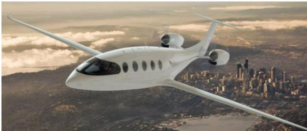
Figure 6 - Eviation Alice, all-electric 9-seats aircraft (source: Eviation)
