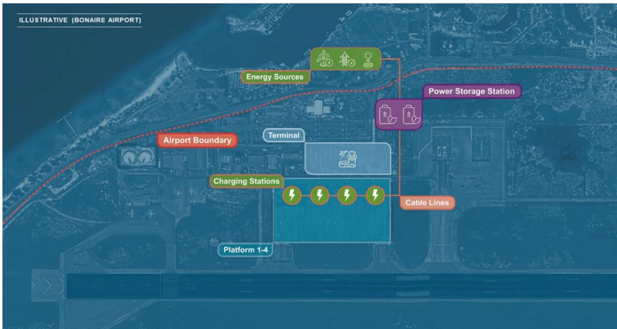
Figure 21 - Overview of the infrastructure required at the airport for electric flight (source: author and underlayer Google Earth)
